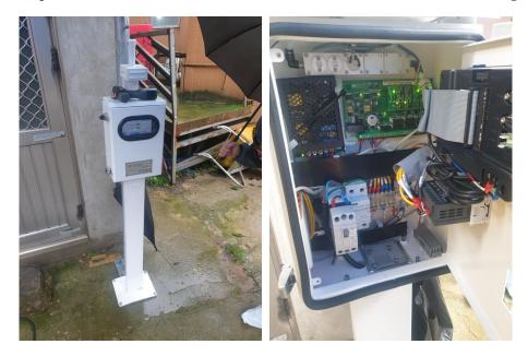
**Figure 2.** The outside and inside of livestock odor management system. The sensor case (outside) must protect the inside, and the inside is composed of a measurement sensor, modules, communication equipment, and power terminal.
