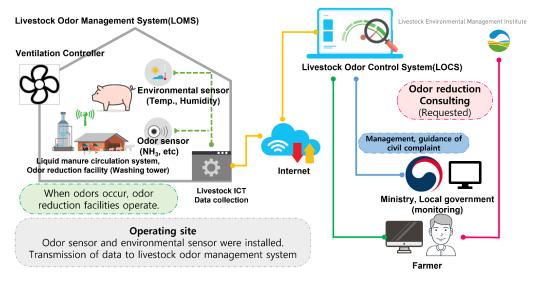
**Figure 1.** Schematic of livestock odor monitoring system. Livestock odor monitoring systems can be divided into LOMS and LOCS. LOMS can be measured by attaching a sensor where ammonia is generated, such as livestock farms. LOCS refers to a system that can receive and check measured data and link the two systems using Internet communication equipment.
